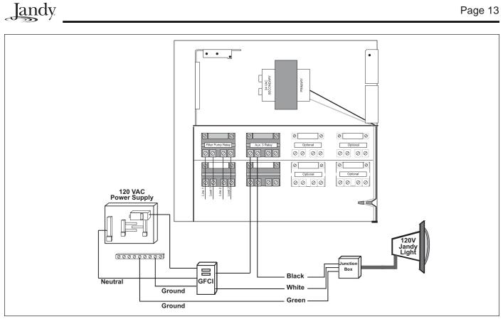
Figure 5. 120-Volt Jandy Pool and Spa Light Wiring Diagram
